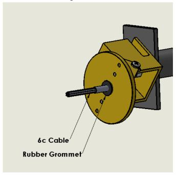
8. Rotate the Mounting Plate to a position that will achieve the desired speaker pan angle. Tighten the screw holding the cube onto the Mounting Plate via the triangle U-Bracket onto the attached locknut to fix the pan angle. Use a 7/16" crescent wrench to hold the lock nut.
