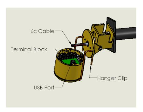
11. Remove Beacon from hanger clips, and remove hanger clips from Mounting Plate. Replace gasket before attaching to Mounting Plate.
