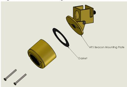
3. Rotate the cube-shaped piece attached to the Mounting Plate so that the large Socket Access Hole in the cube is unobstructed. Insert provided threaded chase nipple through the large hole in the cube and into the small hole on the other side.
