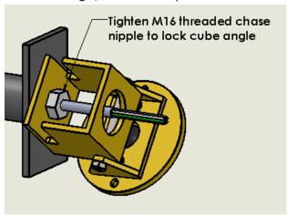
6. Pull wire from chase nipple so that approximately 5" protrudes beyond the socket access hole in the cube.
