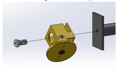
5. Rotate the cube to the desired speaker tilt angle, then tighten chase nipple onto the cube through the large access hole using 7/8" or 24mm open ended crescent wrench.
