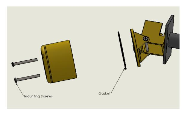
12. Mount APS Beacon to Mounting Plate using the provided %-20 x 3-1/4" PHP screws through the two mounting holes on the front of the Beacon and into the threaded holes on the Mounting Plate.
