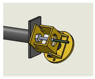
7. Flip Mounting Plate downward so that its center hole sits in front of the open bottom end of the cube. Route the 6c cable out of the open bottom end of the cube and through the rubber grommet in the center of the Mounting Plate
