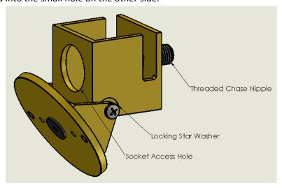
4. Run 6c cable from wire chase hole through the threaded chase nipple.
