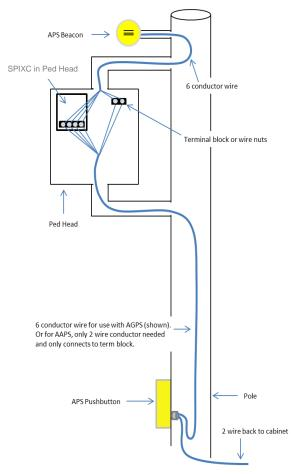
Figure 2. Beacon wiring diagram
