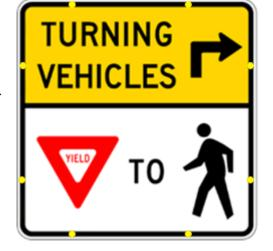
The Turn Lane Pedestrian Indicator (TLPI) provides a visual warning indication to drivers that the intersection is active with pedestrians who are legally crossing the street during the walk cycle in one or more locations that are potentially in a collision path with an automobile. The visual warning only becomes active after a pedestrian has pressed or waved at an APS or PPB.
