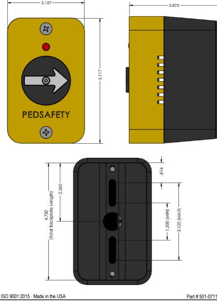
The Guardian Mini 4-Wire Accessible Pedestrian Station (APS) comes ready to install out of the box. A four-conductor cable connects the Signal Power Interface (SPI) in the pedestrian signal head, now 48VDC compatible, to the pedestrian station while your standard field wires run from the button to the cabinet. The housing, crafted from solid 6061 T6 AL, injection-molded thermoplastic, and stainless-steel materials, is virtually vandal-proof.
